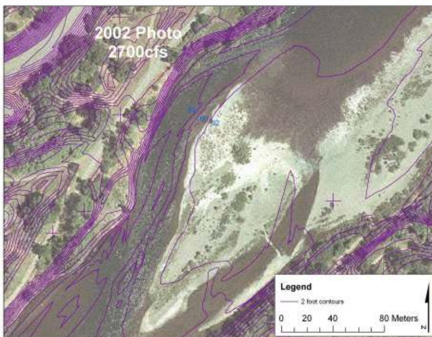
Figure 2-19 Bathymetric contours used to determine the 1.2m (4ft) estimated thickness of the island.
