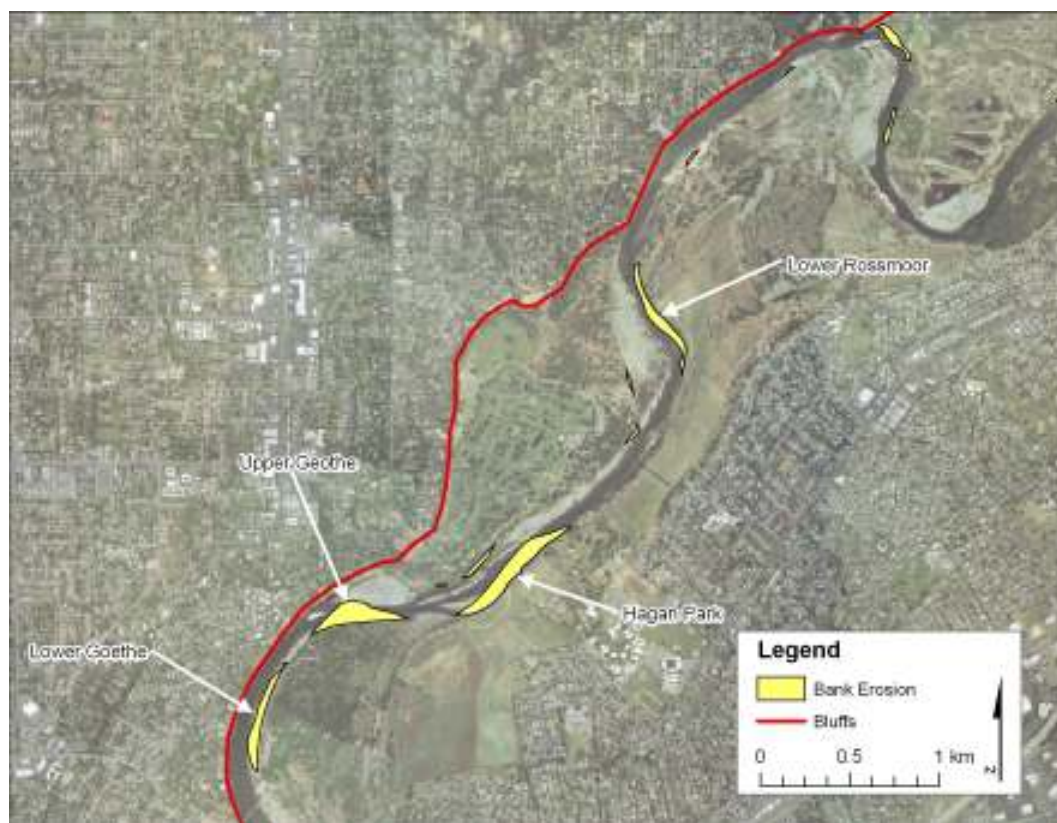
Figure 4-2 Locations of significant bank erosion in reach 3 of the LAR. The location of the bluffs to the north are indicated.
