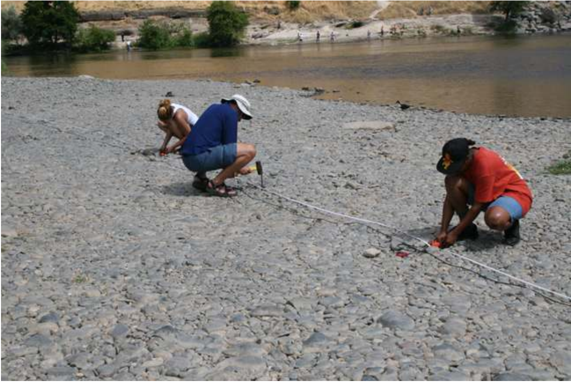
Figure 6-2 Installation of the geophone array. The geophones were secured to 0.3m long rebar pounded into the gravel to ensure good coupling between the geophone and gravel.
