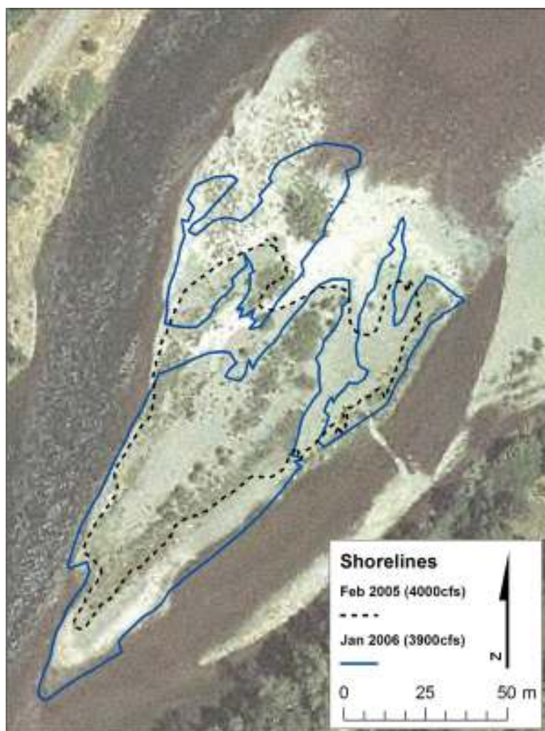
Figure 3-2 Changes in the shorelines during the 36 tcs event of December 2005 to January 2006. Gravel was deposited on the downstream end (lower left) of the bar and two small channels were incised in the gravel bar.
