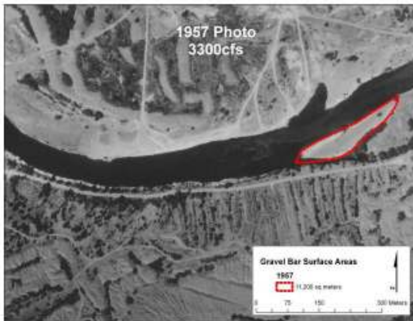
Figure 2-14 Georeferenced photo of Sailor Bar from 1957. The dashed line identifies the likely source of the sediment that forms the island in the 2002 photo (Figure 2-15).
