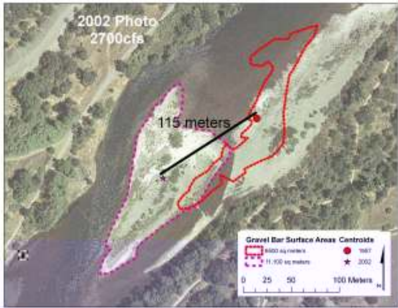
Figure 2-18 Georeferenced photo of Lower Sunrise from 2002. The dashed line on the left shows the modern location of the island. The surface area of the two bars and the distance between the centroids were measured.
