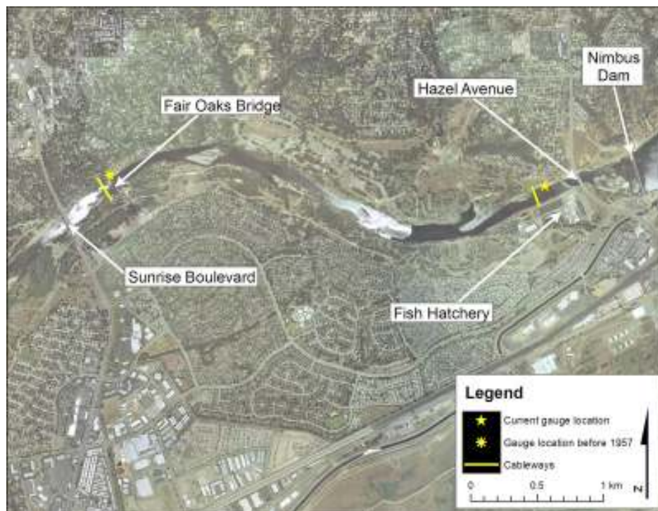
Figure 3-11 Location of Fair Oaks gauge. Prior to 1957 it was located near the Fair Oaks Bridge. The modern location is Near Hazel Avenue.
