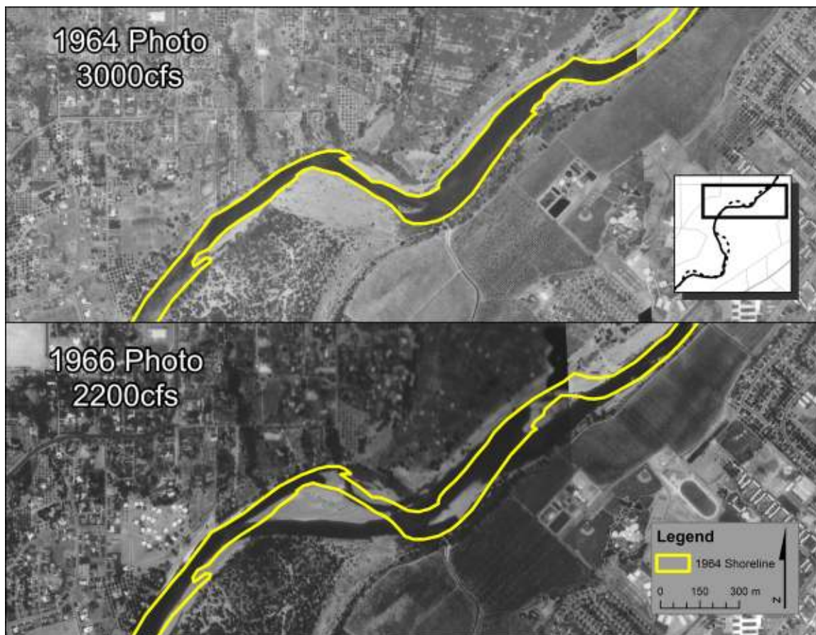
Figure 2-4 Aerial photos showing the channel changes that occurred between 1964 and 1966 between Goethe and Ansel Hoffman Parks. A peak flow of 115,000cfs in 1965 is likely responsible for the straightening of the channel.
