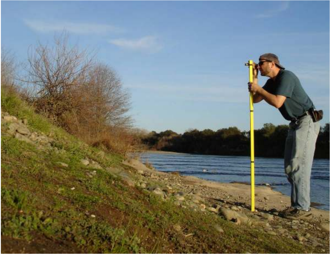
Figure 4-6 Bank heights were measured using a Jacob's Staff and hand level. Black marks on the staff are 50 cm apart.
